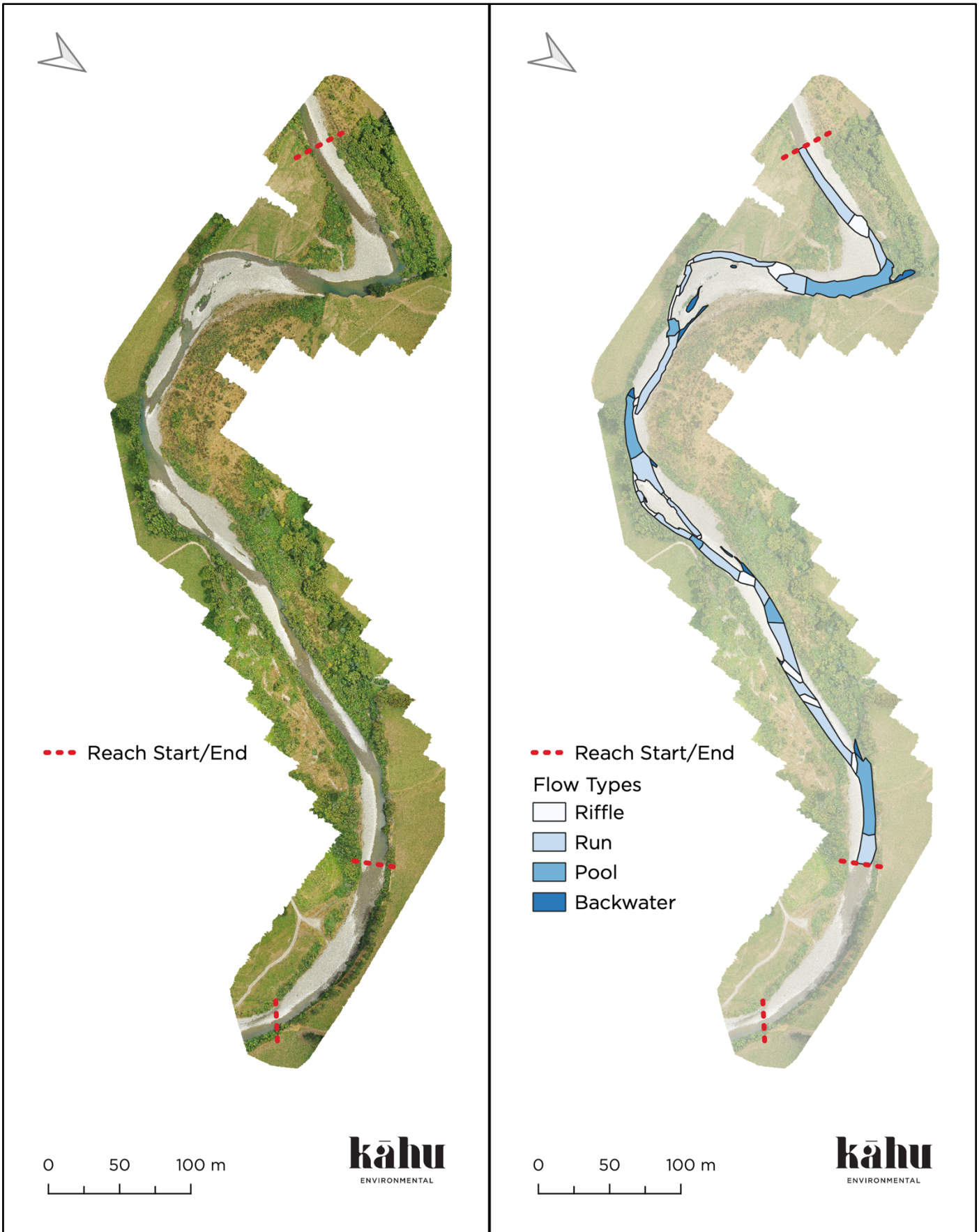
Figure 5: Upstream control reach aerial orthophoto (left) and mapped flow types (right). The start of the downstream (gravel extraction) reach can be seen at the bottom of the images.
