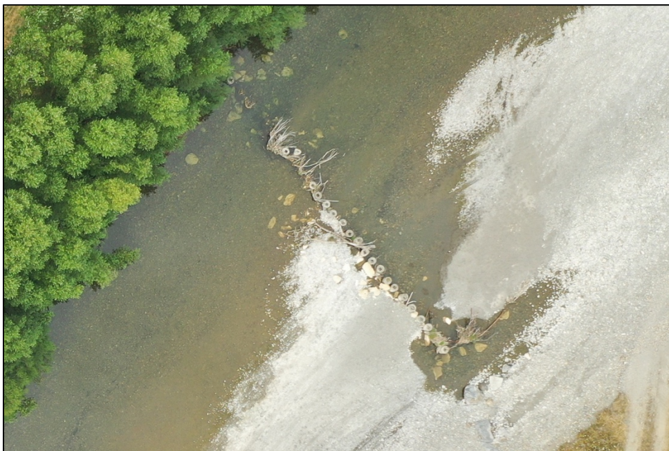
Figure 4: Grade control structure in the upstream control reach with flattened gravel beaches suggesting engineering works or gravel extraction has recently occurred.
